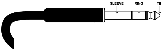
Figure B. Stereo Jack Plug Connections
